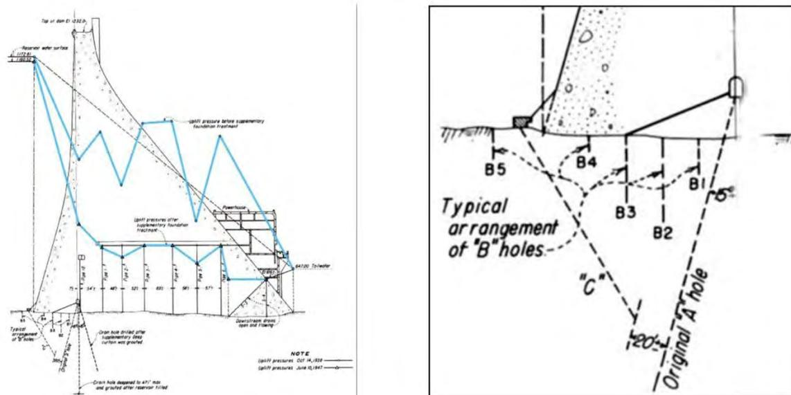
**Figure 3. Left diagram shows blue profiles of uplift pressures measured between 1939-1947, before and after post-construction grouting (Simonds, 1953 and Rogers, 2010). Right figure is an enlargement of network of grout holes drilled beneath the dam's upstream heel.**
