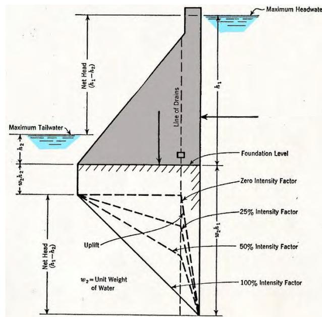
FIG. 1.—DIAGRAM OF UPLIFT INTENSITY WITH VARIOUS FACTORS
