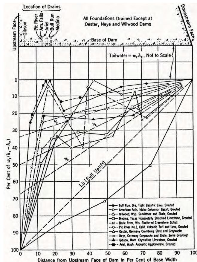
**Figure 7. Observed uplift pressures under 10 gravity dams founded on rock foundations. Note the very high values recorded at Oester Dam in Germany, which were greater than 100% (full uplift). This dam is founded on crumbling slate and greywacke, whose particles may be clogging fissures, joints, and other discontinuities.**
