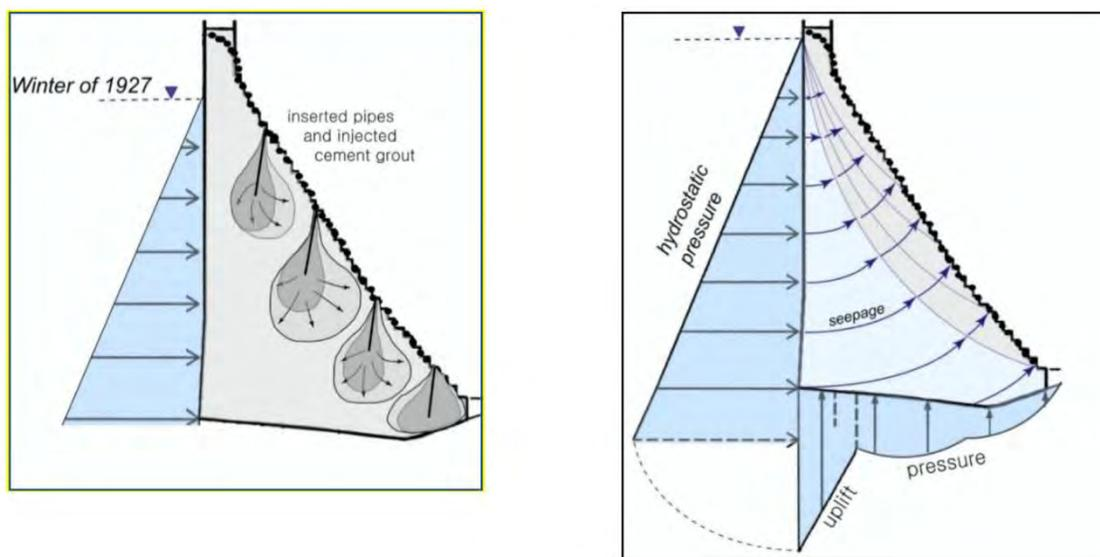
**Figure 1. Left pane depicts the grouting of the transverse shrinkage cracks in the maximum section of the dam in early 1928. Right pane shows the likely impact of the 10 uplift relief wells beneath the main dam, prior to caulking of the transverse shrinkage cracks.**
