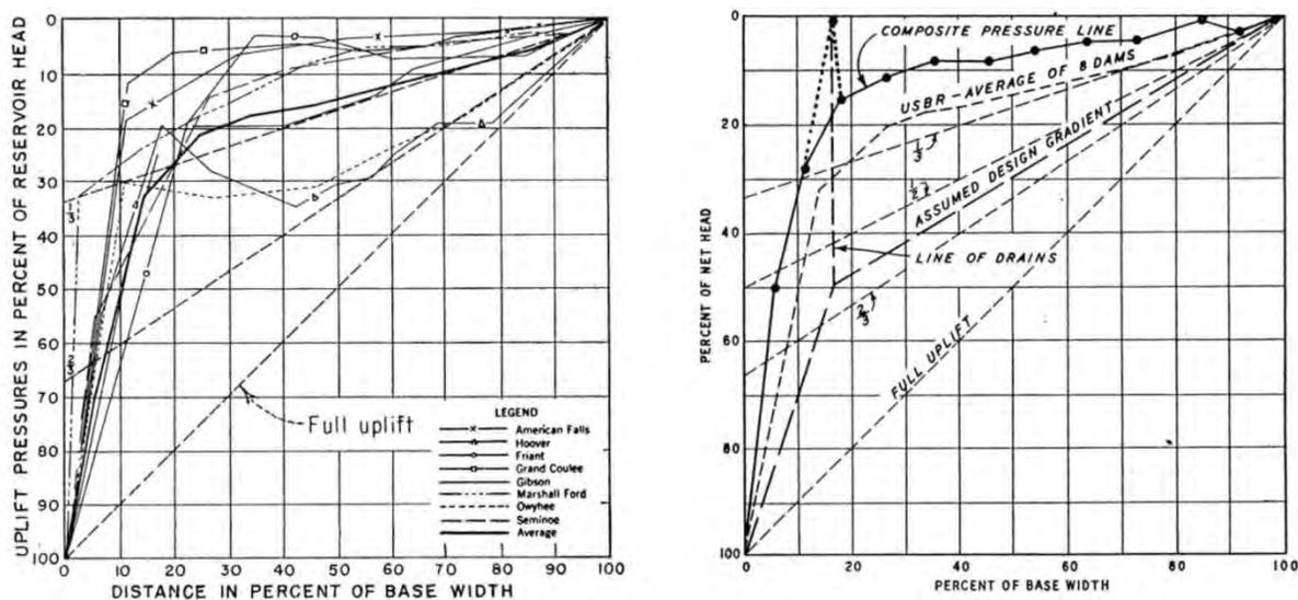
**Figure 8 (left) presents uplift data for Reclamation's largest dams compiled by Keener (1949), with Hoover and Owyhee Dams yielding the highest values. Figure 8 (right) shows the composite foundation uplift intensity for TVA's four highest dams and Reclamation's average line (from Subcommittee, 1952).**
