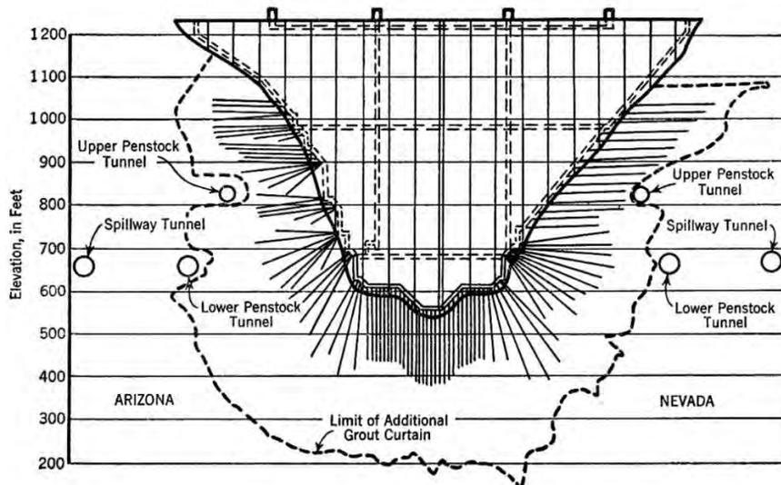
**Figure 4. Profile of dam centerline showing the extent of original grout curtain and that of the deepened grout curtain, installed from 1938 to 1947, shown by dashed line (from Simonds, 1953).**
