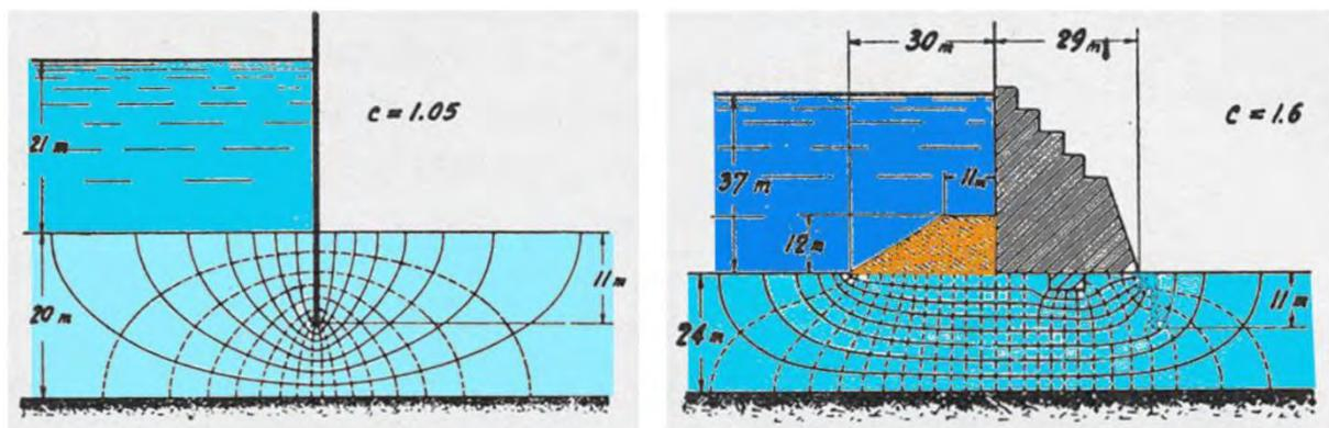
**Figure 2. Seepage nets presented by Terzaghi (1929) for a bulkhead cutoff wall (left) and for a masonry concrete dam with an upstream toe berm. Flow nets allow a rational means of estimating uplift pressure in porous unconsolidated materials, like alluvium.**
